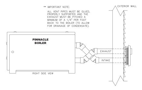
Figure 5.5: PI-399 Sidewall Venting with 4" Pipe (Stainless Steel Vent Kit).
