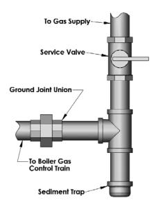
Figure 4.1: Gas Supply Piping - Sediment Trap
