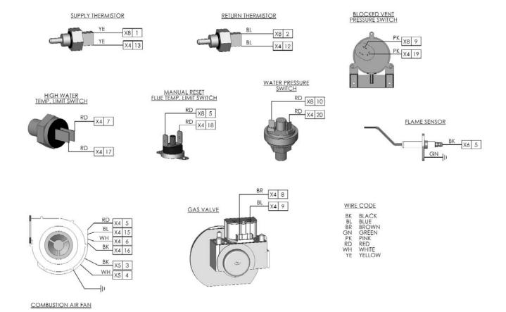
Figure 6.4: Component Wiring
