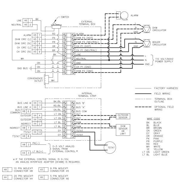
Figure 6.1: Wiring Connections to Boiler Junction Box
