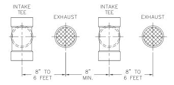
Figure 5.2: Multiple Pinnacle Vent Spacing
