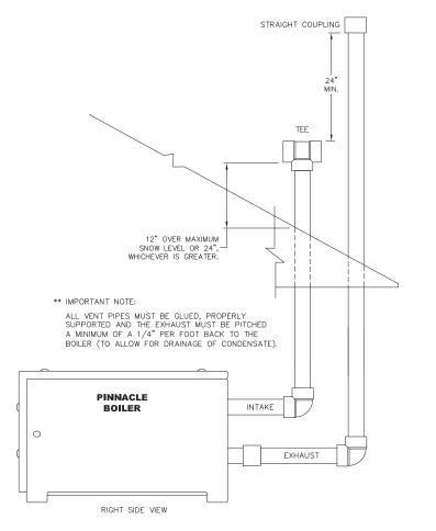
Figure 5.6: PI-399 Vertical Venting with 4" Pipe.
