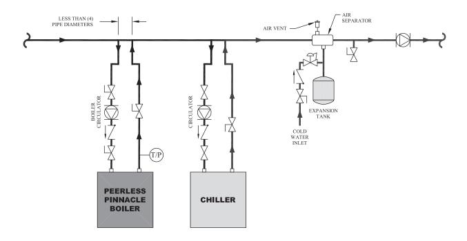
Figure 3.8: Boiler in conjunction with a Chilled Water System
