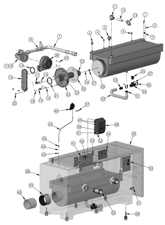
Figure 11.1: Pinnacle P399 Repair Parts
