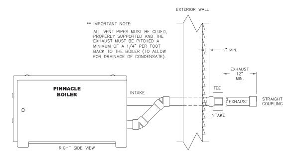
Figure 5.4: PI-399 Sidewall Venting with 4" Pipe (Air Intake and Exhaust on the same Elevation).
