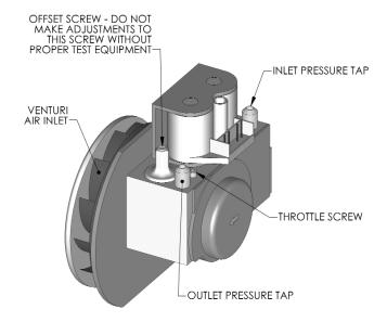
Figure 4.2: Gas Valve/Venturi PI-399
