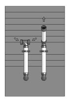
Figure 5.7: Sidewall Venting Below Grade
