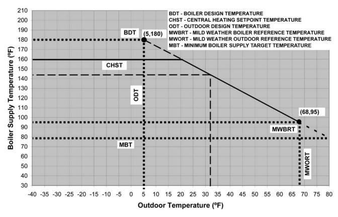
Figure 6.6: Central Heating Curve (Factory Defaults)
