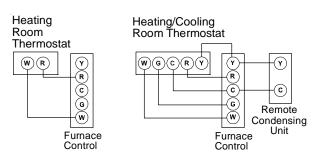
Typical Field Wiring (24 VAC Control Circuit)
