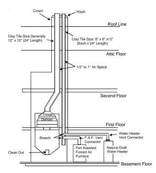
Typical Multiple Flue Clay Tile Chimney
