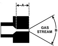
The length of Dimension "A" determines the angle of Gas Stream "B".
