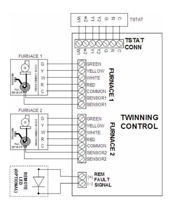
FURNACE TWINING KIT - FTK04 (UTEC Control Board) This wiring diagram is for reference only. Not all wiring is as shown above. Refer to the appropriate wiring diagram for the unit being serviced. (For use only with 80% or 90% Single-Stage Furnaces)
