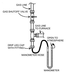
Measuring Inlet Gas Pressure (Alternate Method)
