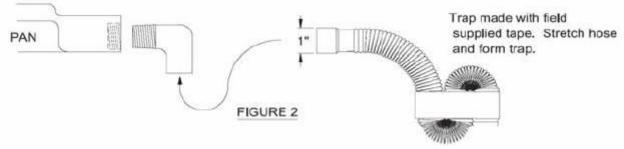
SLIP 1" ID SECTION OF HOSE ONTO 90 DEGREE DRAIN FITTING.
