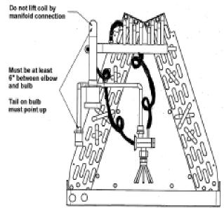
Revolv coils use the Chatleff type distributor body that accepts a screw on TXV or accepts a Chatleff style piston. All metering devices, both pistons and TXVs, have a relationship to the outdoor unit. The proper metering device allows for proper system operation but does not increase or decrease the capacity. The system capacity is determined by the relationship of the indoor-outdoor combination and air flow.
