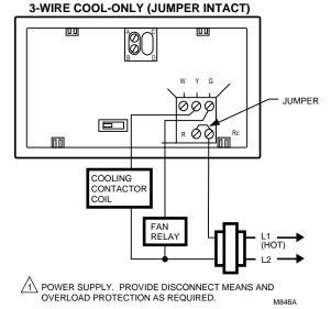
Fig. 6. 3-wire cool-only application (jumper intact).
