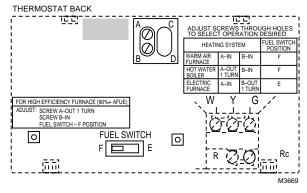
Fig. 9. Back view of thermostat.
