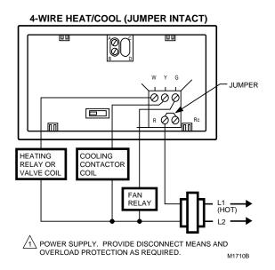
Fig. 7. 4-wire heat/cool application (jumper intact).
