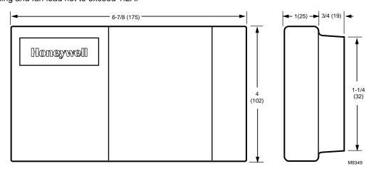
Fig. 1. T8112 dimensions in in. (mm).
