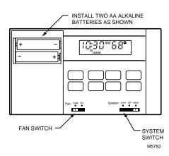
Fig. 11. Installing batteries.
