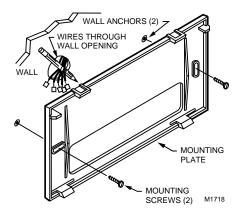
Fig. 2. Mounting plate installation.
