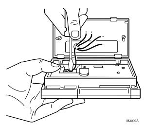
Fig. 4. Holding thermostat while installing.
