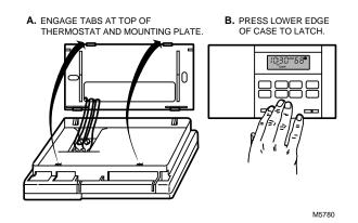
Fig. 12. Mounting thermostat on mounting plate.
