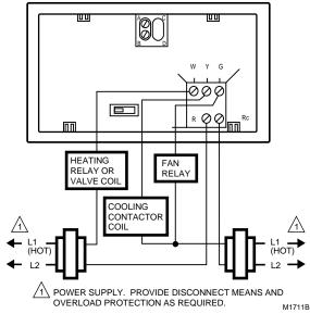
5-WIRE HEAT/COOL (JUMPER REMOVED)
