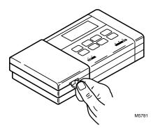
Fig. 10. Removing battery door.
