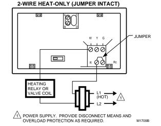
Fig. 5. 2-wire heat-only application (jumper intact).
