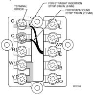
Fig. 3. Wiring connections.
