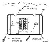
Fig. 2. Mounting wallplate to wall.
