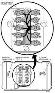
Fig. 4. Restrict wiring to shaded area.
